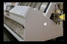
The open type body enables easy access to the cleaning positions.
