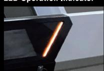
An LED operation indicator on the front of the NIRAMI allows operators to see the machine status at a glance.
