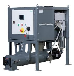
*The K7 Continuous Seed Treater is suitable for small and mid sized plants with its variable capacity of up to 6.3 tons of seed per hour and dosing rates from 100 ml to 2.4 litres per 100 kg seed.*
