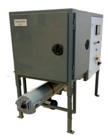
The R15 Continuous Seed Treater is a machine designed for seed plants with a need for treatment of cereals, corn, peas, soybeans, OSR, cotton, sunflowers, etc with a capacity between 5,4-13,5 tons per hour.
