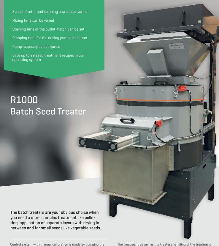
treating liquid to a separate measuring glass in a closed system. When the settings and calibrations are made, the machine run continuously. It is also possible to get an even more sophisticated supervision system with a larger size touch screen. By adding the ULD Control system to your system you get an automatic calibration of dosage rates for both liquids and powders, and a continuous control of dosage rates.
