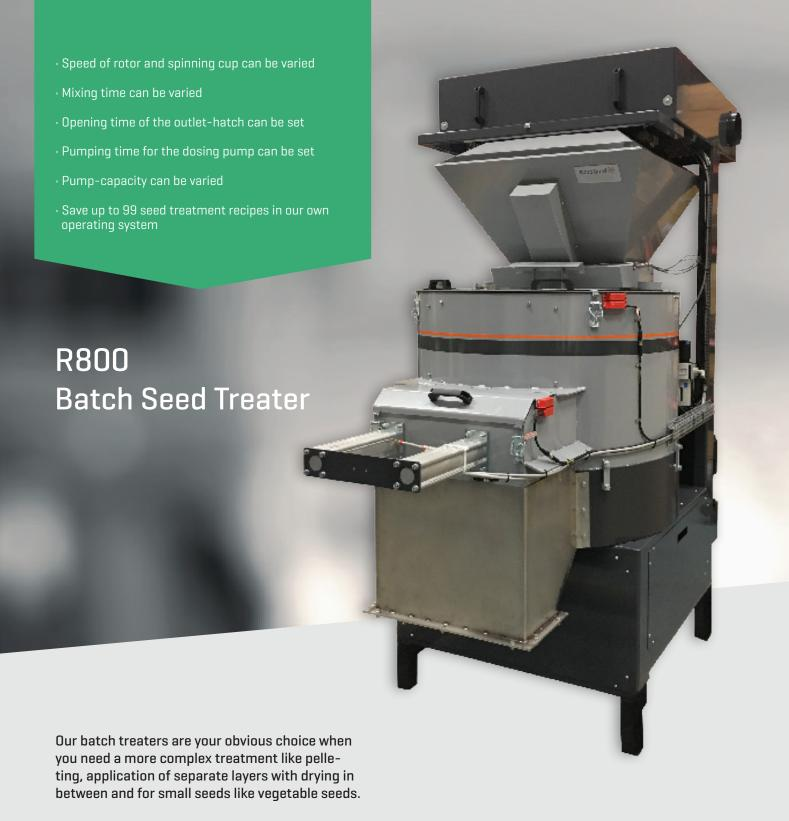
Control system with manual calibration is made by pumping the treating liquid to a separate measuring glass in a closed system. When the settings and calibrations are made, the machine run continuously. It is also possible to get an even more sophisticated supervision system with a larger size touch screen. By adding our ULD Control system to your system you get an automatic calibration of dosage rates for both liquids and powders, and a continuous control of dosage rates.
